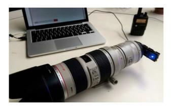
Yesterday I succeeded in hacking a 2006 design awarded Logitech Ultra Vision webcam to fit on my Canon EF 70-200mm EF USM II lens. With a 2x extender, the 1.3 MP 5mm sensor translates this camera in a huge 2800mm tele lens unit! This is needed to get a good view from the relay station to the iSemaphore, apx. 1km away.
