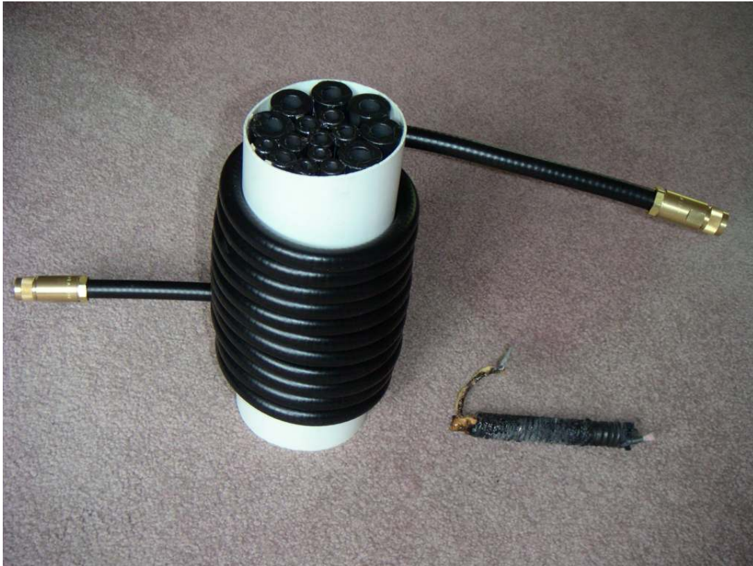
Figure 5: At upper left, a coaxial common-mode choke made by winding Heliax® LDF4-50 semi-rigid coax on a cylindrical core containing 15 lbs. of ferrite beads. At lower right, the charred remains of a Radio Works T-4 Line Isolator like the one that the Heliax-wound choke replaced.
