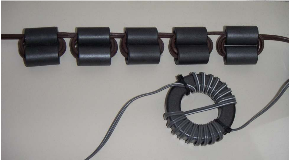
Figure 17. Above, a common-mode choke in the 2 \times AWG 18 zip-cord of a 120-VAC, 6-A, extension cord. This is a series string of five binocular cores each wound with 2 \frac{1}{2} turns. Below, a common-mode choke in the thin, 2 \times AWG 24, zip-cord of a wall wart. This is a 5943003801 toroid wound with 17 turns. The winding is split to increase the separation between its ends, to reduce capacitance and improve high-frequency performance. In practice, the improvement is slight.
