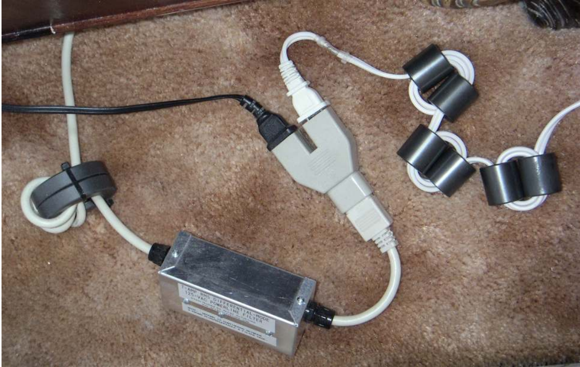
Figure 12: 7-A, 115-VAC, two-stage, L-C, difference-mode EMI filter by W3NQN, with ferrite-toroid and -bead common-mode chokes added.
