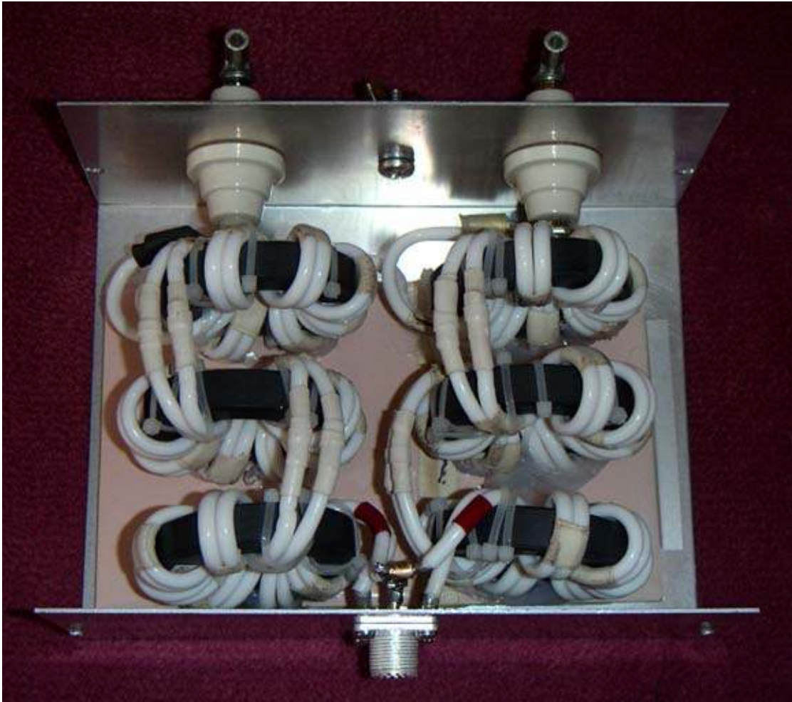
Figure 6: Homebrew 4:1 current balun for 160 through 10 meters, built to handle 15 kW with SWR = 1, and 1.5 kW with SWR = 100.
