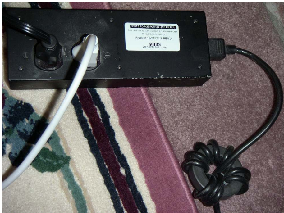
Figure 9: Potter 12-A, 115-VAC, difference-mode EMI filter in box with duplex outlet, bought at hamfest for $10. (Ferrite toroid on line cord not included.)
