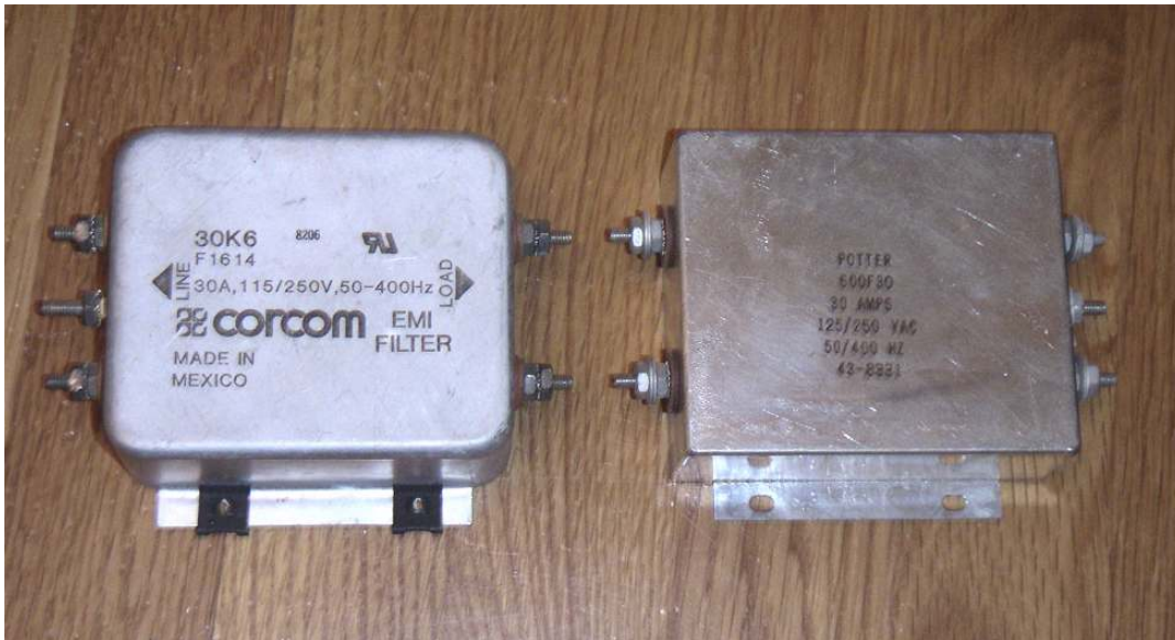
Figure 8: Corcom and Potter, 30-A, 115/250-VAC, difference-mode, EMI filters bought at hamfests for $5 each.
