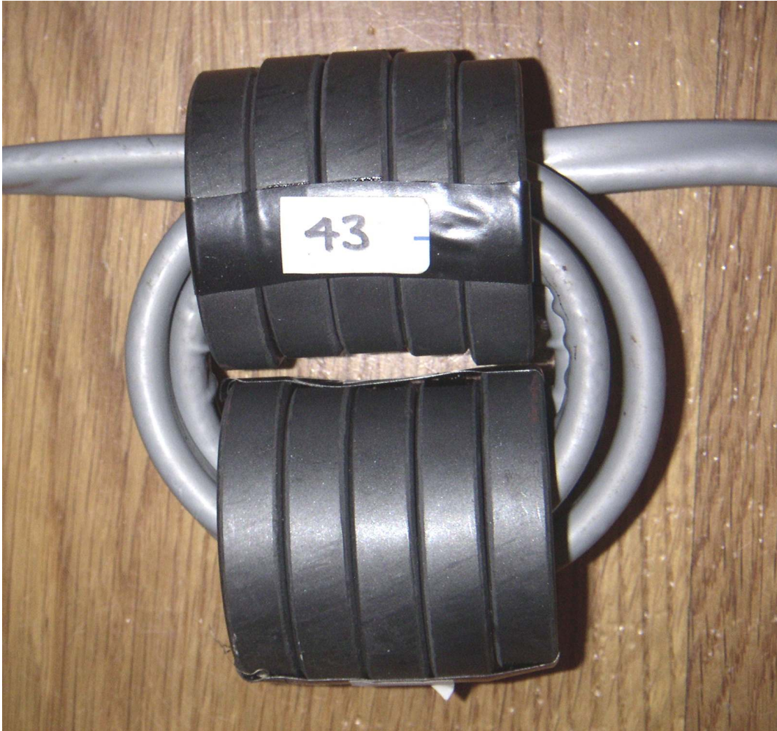
Figure 13: Common-mode choke for a 2 \times AWG 4, DC power cable, formed by threading the cable 3\frac{1}{2} times through a binocular core formed by two stacks of five Fair-Rite p/n 5943003801, mix-43, “ring” toroids.
